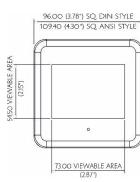
96 × 96 DIN 4.3" x 4.3" ANSI Front of Panel19.9mm (0.78") Rear of Panel 78.3mm (3.00") IP52 (front panel), IP30 (rear) Panel Mounted DIN96, ANSI DIN 96 92mm x 92mm square ANSI C39.1 4" round
